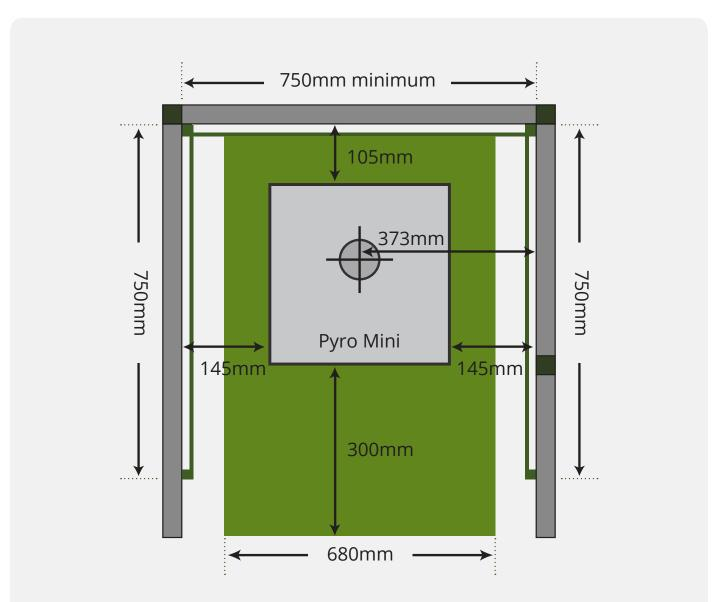
Side screens will only need to protect the combustile lengths of the built wall up to **750mm**. If wall is shorter, the screen will be shorter.
