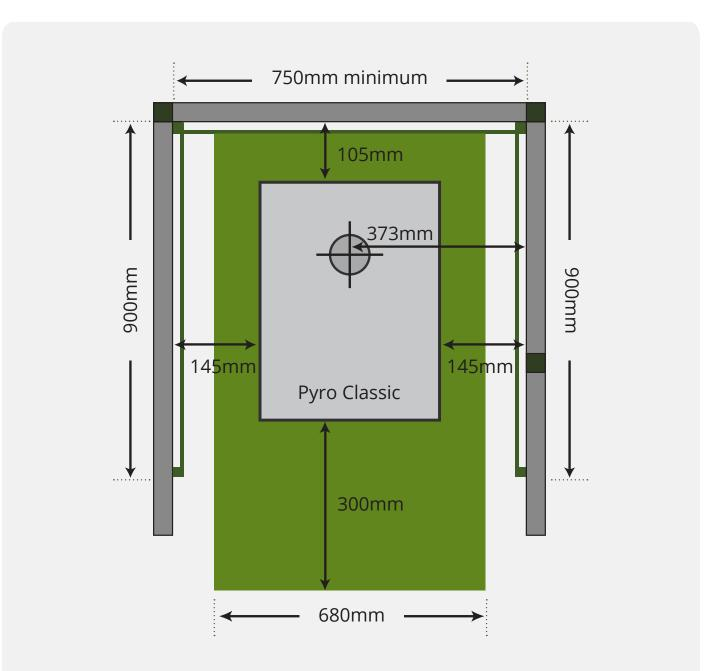
Side screens will only need to protect the combustile lengths of the built wall up to **900mm**. If wall is shorter, the screen will be shorter.
