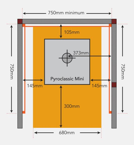
Side screens will only need to protect the combustile lengths of the built wall up to **750mm**. If wall is shorter, the screen will be shorter.
